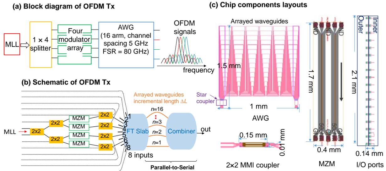
Fig. 2. (a) Block diagram and (b) schematic of the 4-channel AO-OFDM Tx PIC using AWG; (c) Layouts of OFDM Tx PIC components include a “u-wave-bend” arrayed waveguides, MZM, 2x2 MMI coupler, and two fiber connector arrays.
