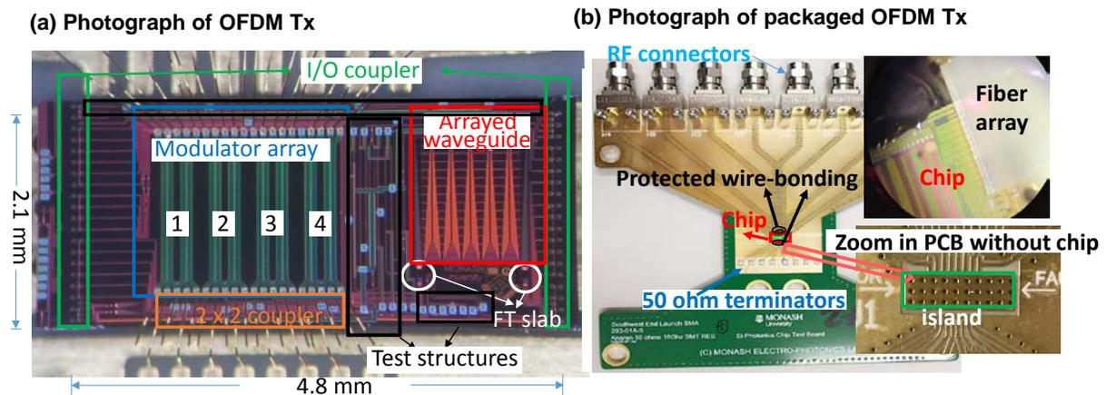
Fig. 1. (a) Photograph of a fabricated AO-OFDM Tx PIC. (b) Photograph of PCB-mounted OFDM Tx.
