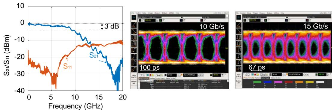
Fig. 4. Normalized electro-optical  $S_{21}$  and  $S_{11}$  as a function of frequency MZM and eye diagrams at 10 Gb/s and 15 Gb/s.
