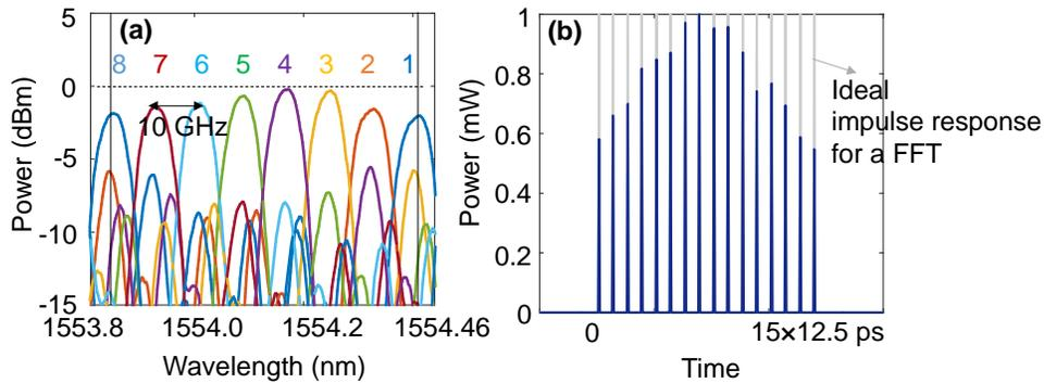
Fig. 3. (a) Spectral and (b) impulse responses of the AWG. (FFT: fast Fourier transform algorithm).
